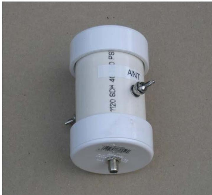
*Figure 14. Completed feedpoint preamplifier*
