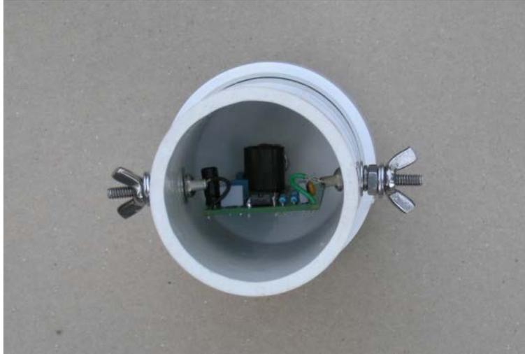
*Figure 13. Mounting of PCB inside PVC pipe*
